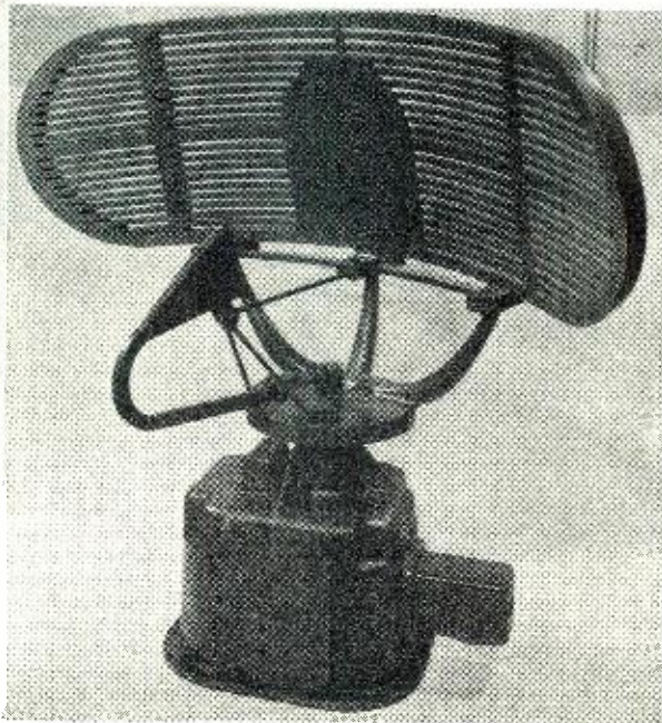
The parabolic reflector in the scanner component of the Sperry Gyroscope marine radar is 48 inches by 18 inches and rotates 360 degrees in azimuth at about 15 revolutions per minute. Contained in the splash-proof box are a driving motor (split-phase ½ horsepower squirrel cage induction motor) and a type 5G synchro generator.
