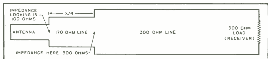
Fig. 4. Method of matching antenna to receiver via a quarter-wave transformer.
