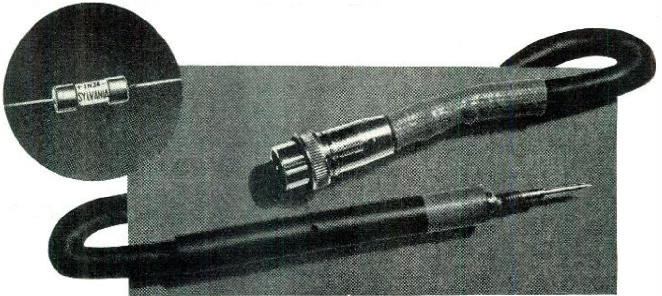
The 1N34 crystal diode when mounted in housing shown makes a convenient test probe.
