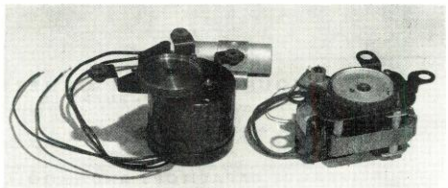
Synchronous motor compared with conventional shaded-pole induction motor.
