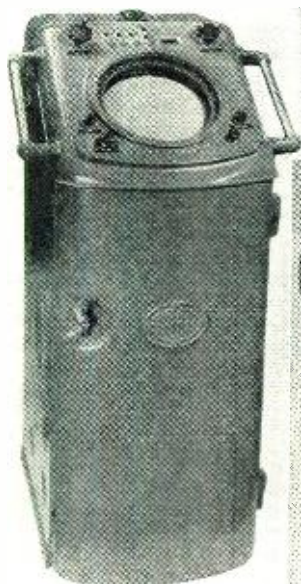
Indicator binnacle of the Sperry Gyroscope set houses 12" PPI and associated controls. Visible are range selector switch, variable range marker, bearing cursor, anti-clutter selector switch, and azimuth scale illumination control.
